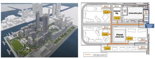
Figure 32: Harumi Flag after completion - bird's eye view and hydrogen supply conceptual schematic.
