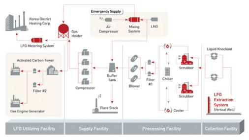
Figure 40: Flow Diagram of LFG Utilization System (Source: Daesung Group website)
