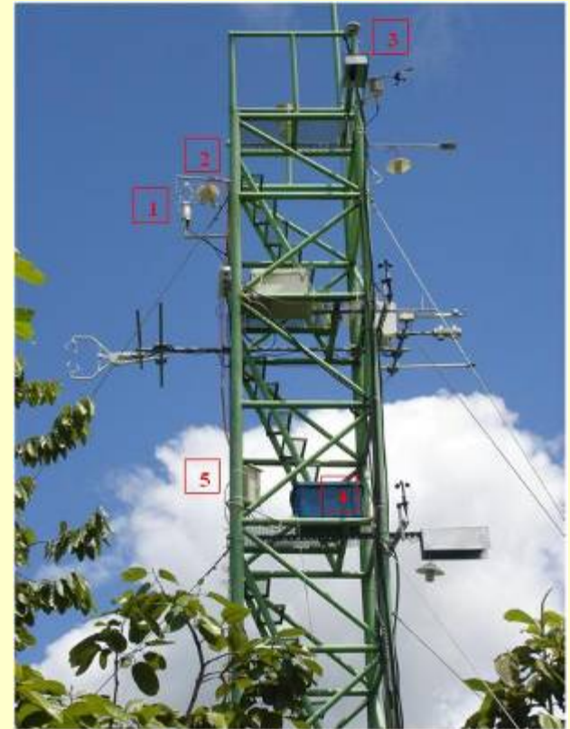
Experimental tower equipped with meteorological instruments in the deciduous tree forest in Thailand for Aerosol Deposition Studies
