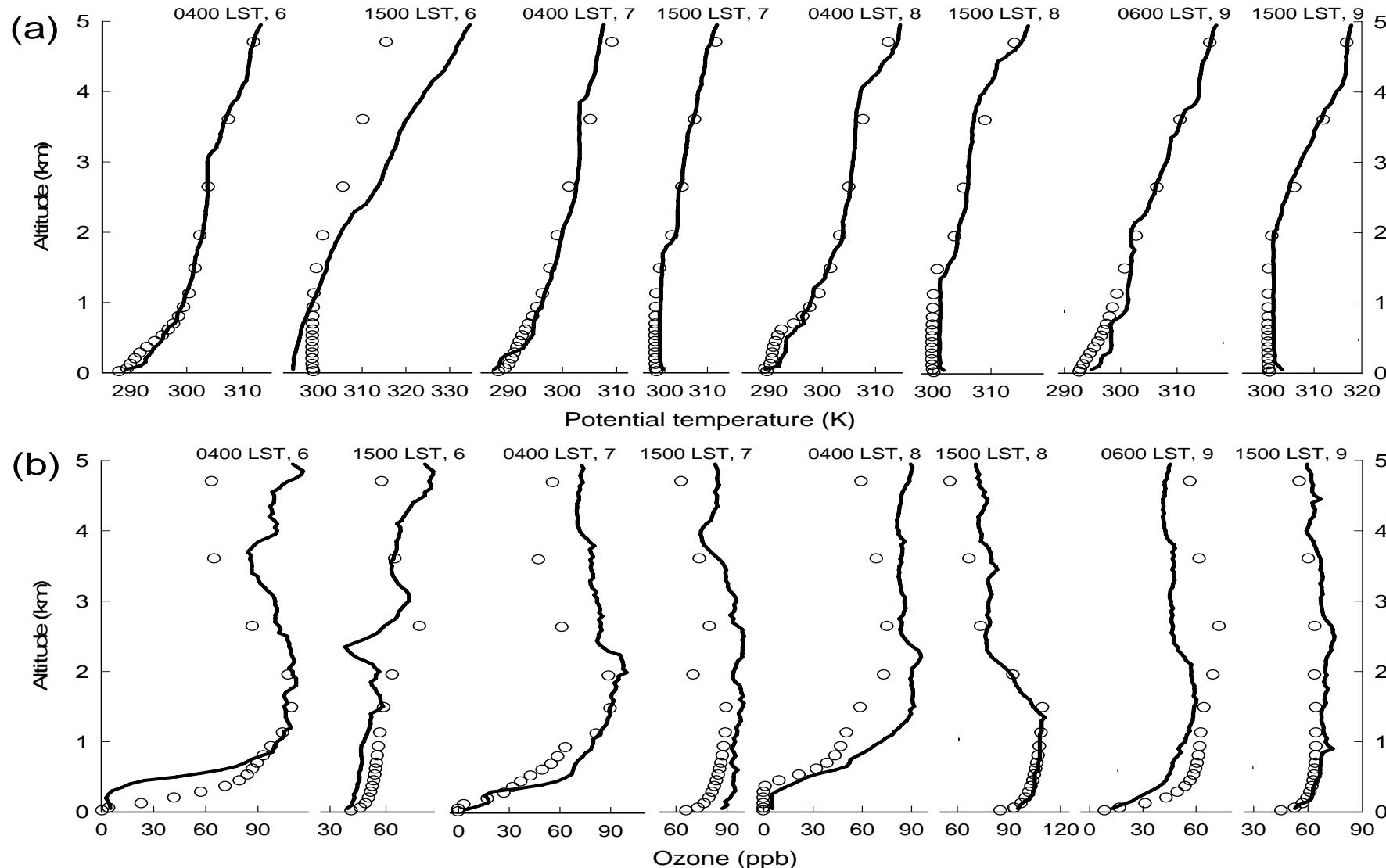
Observation (line) vs. Simulation (circle) for (a) Potential Temp. (b)  $O_3$
